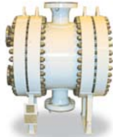
2135 kW 2 nd Stage Suction Cooler (sweet natural gas) operating on a Gas Production Platform, PSHE 7HH-256/1/1 (55 bar design, titanium plates, duplex shell)
