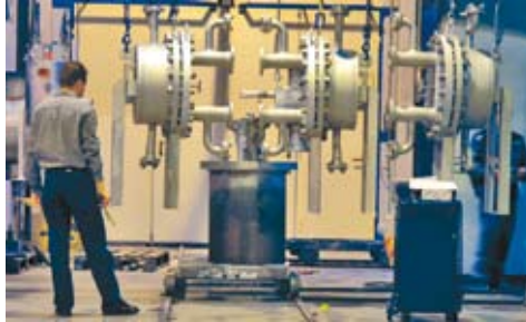
480 kW Raffinate Stripper Bottoms Cooler, PSHE 5HH-148/1/1
